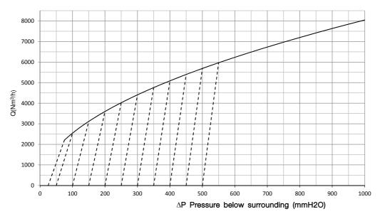
Nominal size: 250mm Volumetric Flow Capacity
