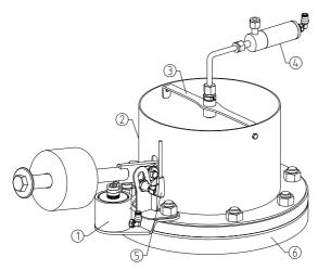
Pos. 1: Force opener: force-opening during valve seat cleaning
