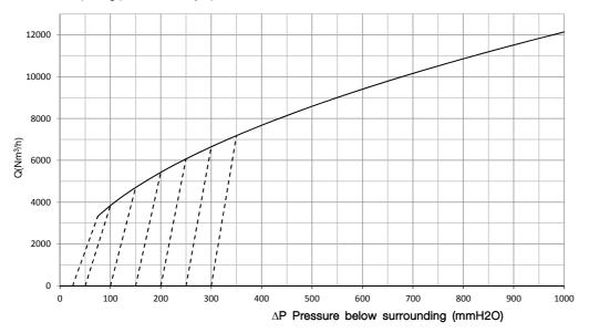
Nominal size: 300mm Volumetric Flow Capacity
