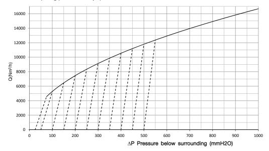
Nominal size : 400mm Volumetric Flow Capacity
