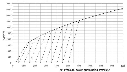
Nominal size: 200mm Volumetric Flow Capacity
