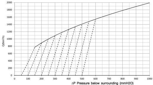
Nominal size: 150mm Volumetric Flow Capacity
