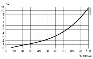
The flow in % of the total flow at a pressure drop of 1 bar.
